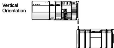
How you orient I/O banks determines which expansion cables you need to connect the I/O banks.
